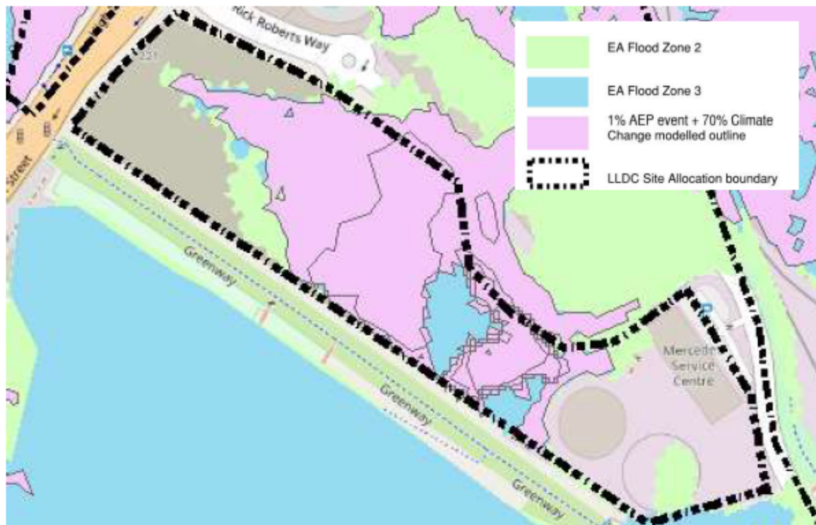
Figure 13 - EA Flood Maps for Planning and flood outline from LBN updated mapping 16 showing the 1% AEP flood extents plus 70% Climate Change for SA 3.6
