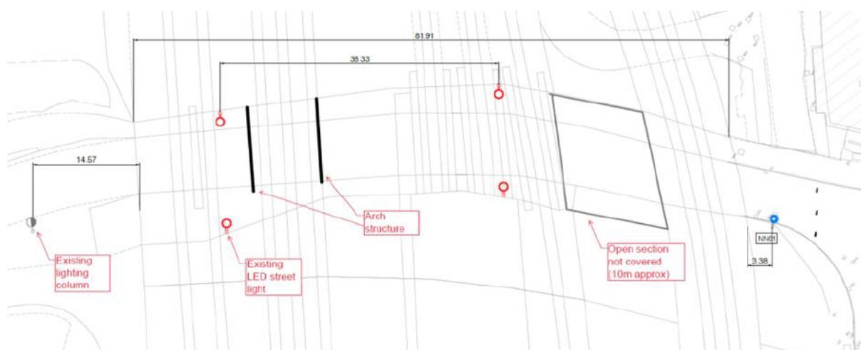
Figure 12 – Sketch of Marshgate Lane Underpass
