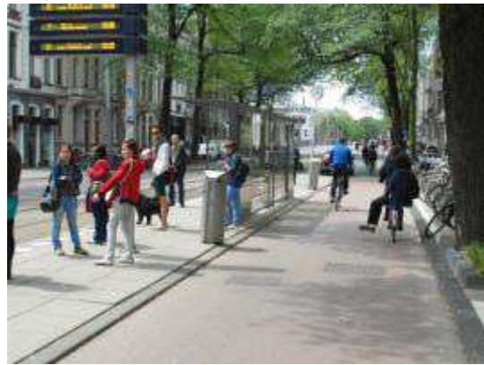
Figure 3.8: Bus Stop Accommodated Within a Flexible Verge
