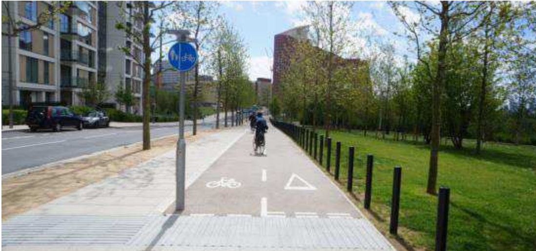
Figure 7.1: Typical streetscape in the Olympic Park with a segregated cycle track within a wide footway
