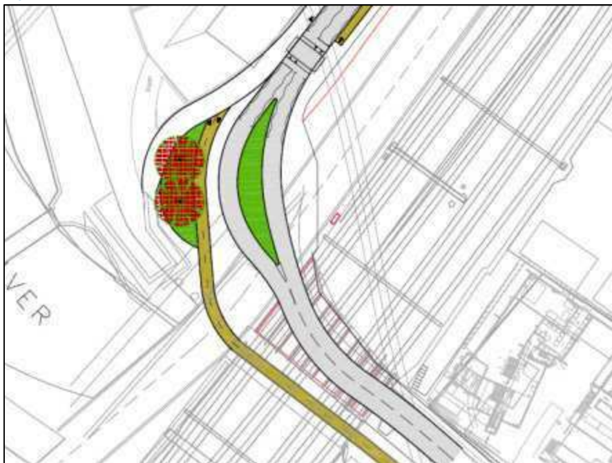
Figure 4.7: Removal of Roundabout on Montfichet Road South
