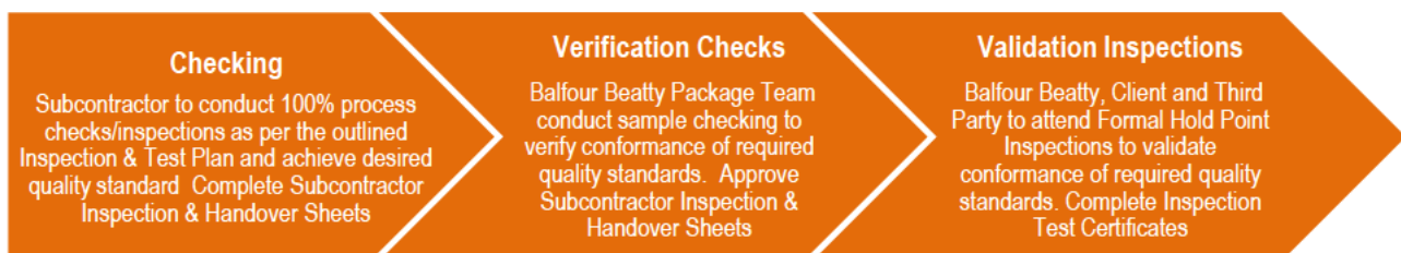
Figure 2: Handover Documentation – Submittal of records supporting Completion Handover: Health & Safety File, O&M, Record Drawings, Assurance Documentation & certificates.
