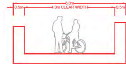
Typical Section at Bridge
