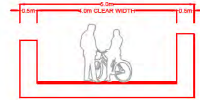
Typical Section at Bridge
