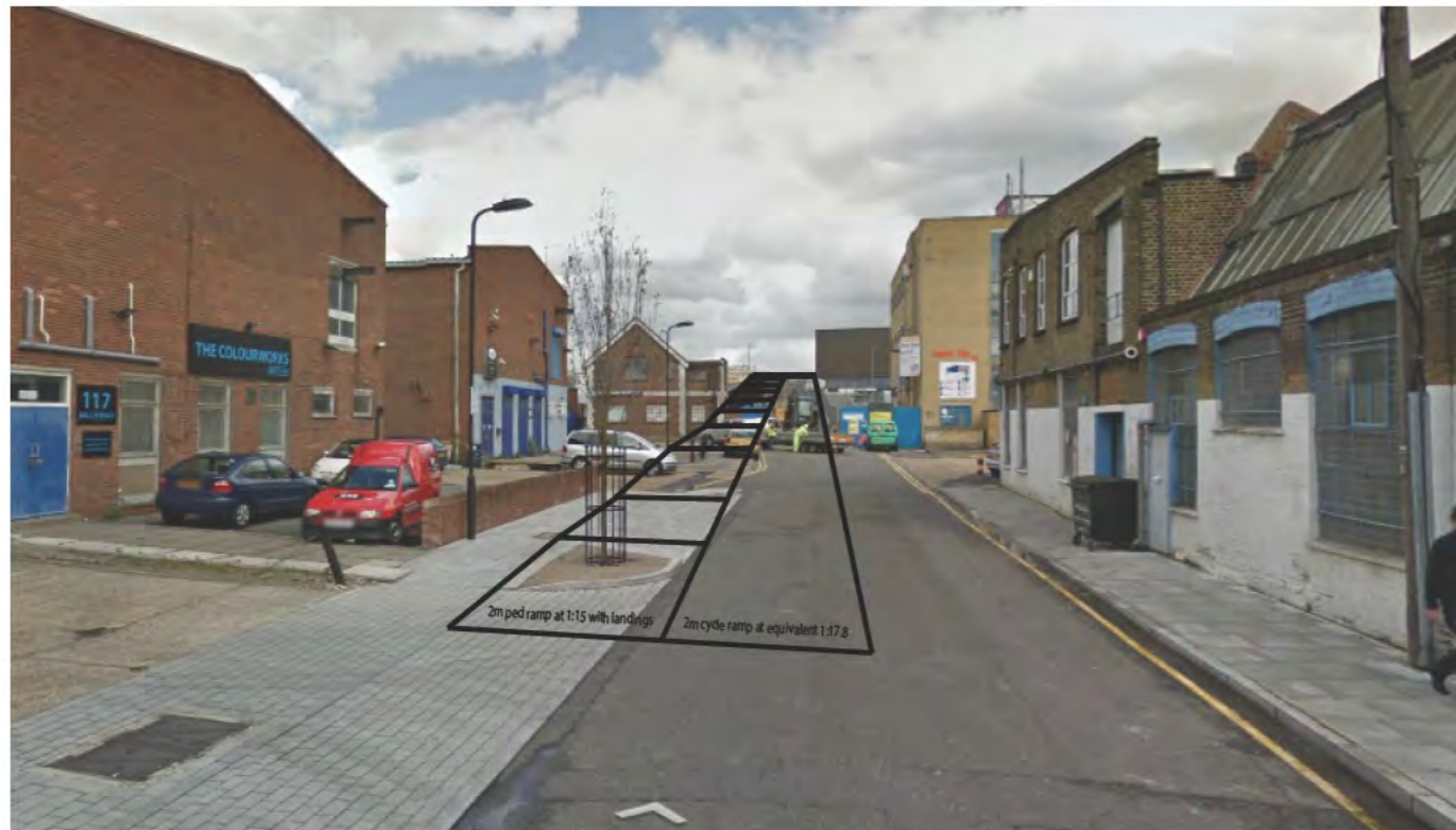
Figure 9.14 - Approximate location and size of 2m wide ped ramp with landings & adjacent 2m cycle ramp for option F
