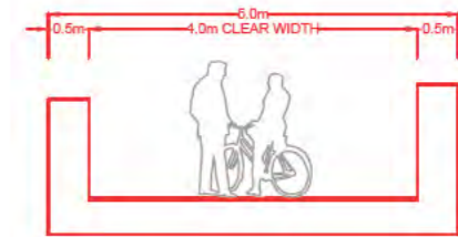
Typical Section at Bridge
