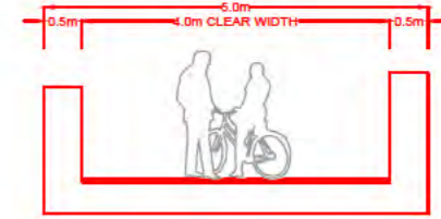
Typical Section at Bridge
