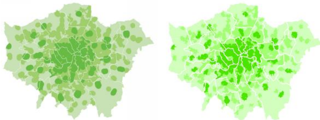
Figure 6: Basic buffer (left) and Network buffer (right) mapping. Both maps use 800m buffers and a 75% predominance of typology. Full map information available in appended Figures
