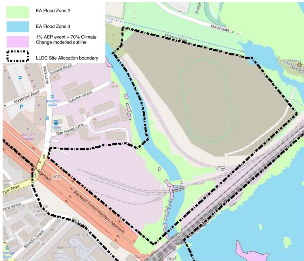
Figure 19 - EA Flood Maps for Planning and flood outline from LBN updated mapping showing the 1% AEP flood extents plus 70% Climate Change for SA 4.5
