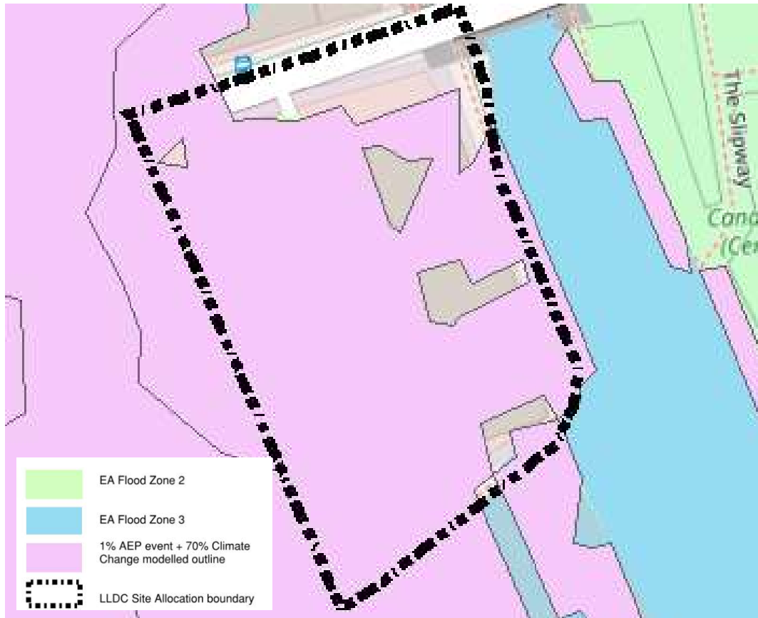
Figure 3 – Updated flood outline from LBN updated mapping 6 showing the 1% AEP flood extents plus 70% Climate Change for SA 1.2
