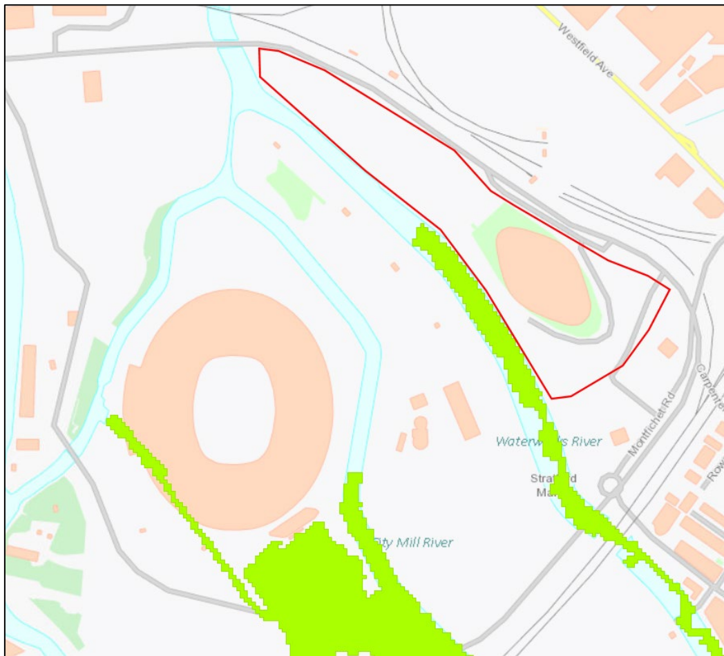
Figure 9: Thames Tidal Breach Modelling Maximum Extents for MLWL for Stratford Waterfront East
