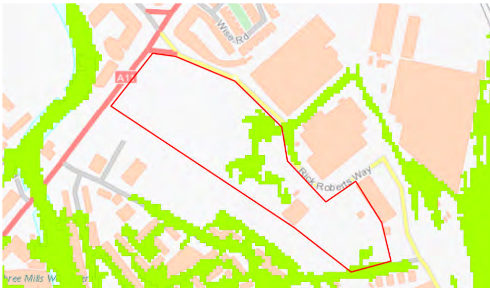
Figure 23 - Thames Tidal Breach Modelling Maximum Extents for MLWL for Stratford Waterfront East
